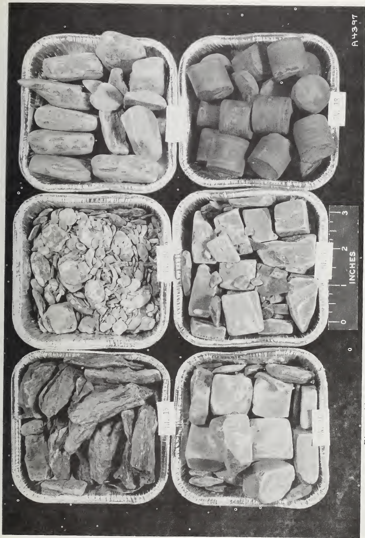
Figure 44. Material remaining after slake-durability testing, TN 13-TN 18.
